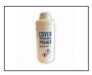
Water-based adhesion primer from Cover Styl', for applying interior films and other films to absorbent surface and difficult to adhere substrates such as untreated wood and plaster. Not intended for smooth surfaces such as furniture panels, glass, smooth painted doors, etc.
