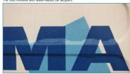
Due to the silicone content in modern car lacquers the adhesion of film can be far from optimal. Film under tension (especially in recesses) is bound to come loose and ultimately be returned for repair or renewal.
