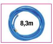
Flexible soft water hose with a length of 8.3 m. Specially designed for high-pressure sprayers such as The WaterBomb (550-WB10). This water hose with an internal thickness of 6 mm, has a reinforced inner core so it can have a pressure of 15 bar. This high quality hose is resistant to pinching, kinking, oils and mild acids and salts.
