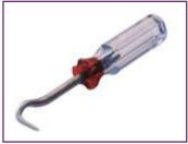
Easy tool for tinting of cars, to get the door rubbers in their proper place again, when they were pushed down while tinting the window.
